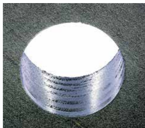
hole exit in unidirectional CFRP hole d = 6.35 mm 單向性的CFRP孔出口 孔徑 = 6.35mm
